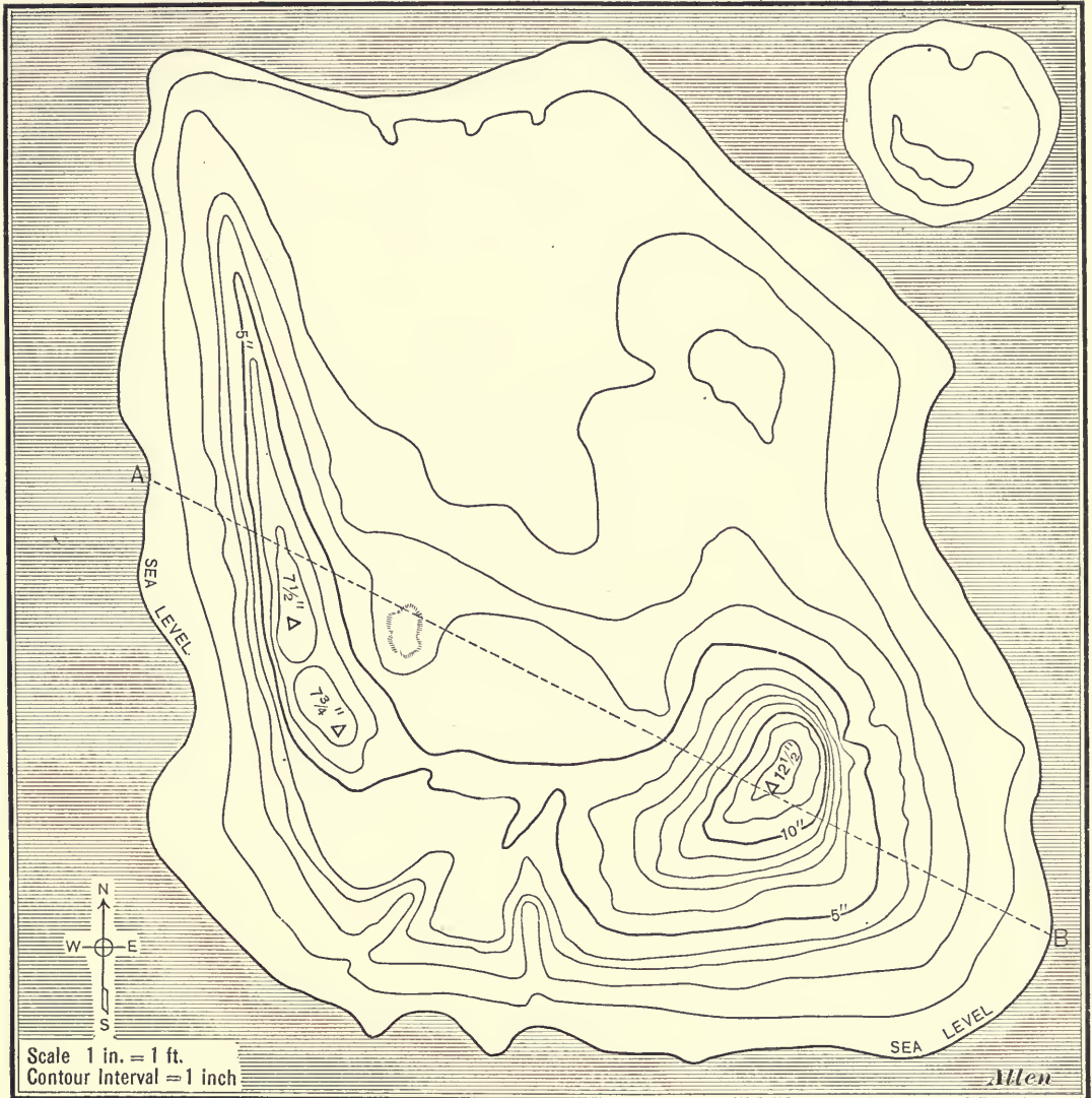
FIG. 15.—CONTOUR MAP OF MINIATURE LAND FORM MADE BY A STUDENT IN PHYSICAL GEOGRAPHY.
